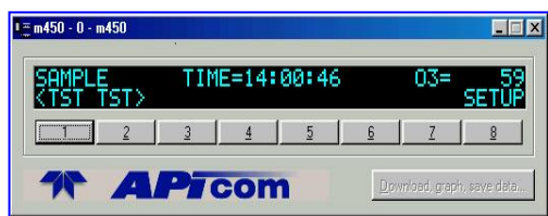
Fig. 8: Display panel of ozone gas meter Teledyne API Model 450H O 3 Monitor
