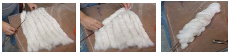
Fig.3 The angle 45 degree laying
