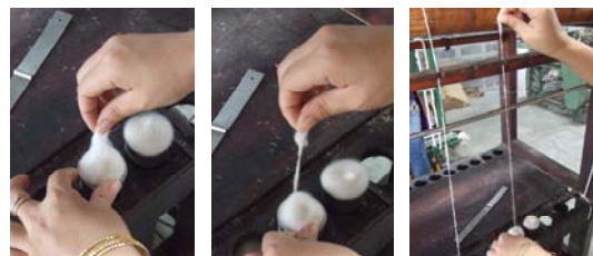
Fig.5 showing about spinning Fancy yarn as SLUB YARN in the longwise laying in GAREBO yarn Tube.
